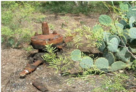
Typical Shut-In Well at Time of Purchase
